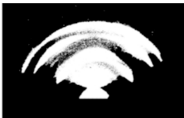
Fig. 1. Electron diffraction pattern of a thin DySb film (fused silica substrate, film thickness of 1.9 mm).
